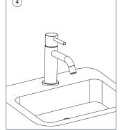
AFTER INSTALLATION, SWING THE OUTLET PIPE FROM SIDE TO SIDE AND TEST WHETHER EACH CONNECTION IS LEAKINGOR NOT.
