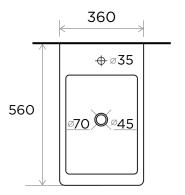
Due to the simplicity of the back-to-wall concept. Installation is achieved by connecting the water inlet/outlet and securing the bidet with the included fixing kit.
