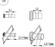
CUT THE STRAIGHT TUBE AND CONNECTING PIPE AS PER ABOVE DRAWING.
