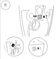
PUT THE PART C INTO THE INSTALLING HOLE ON THE PAN.
