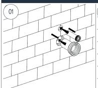
FULL INSERT THE STRAIGHT TUBE INTO CISTERN FLUSHING OUTLET AND DISCHARGING OUTLET.
