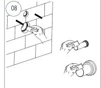
APPLY LUBRICANT ON JOINT SURFACE OF STRAIGHT TUBE AND CONNECTING PIPE
