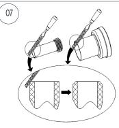
POLSHING THE CUTTING SURFACE TO GET CHAMFER ANGLE AS PER DRAWING AND DEBURRING.
