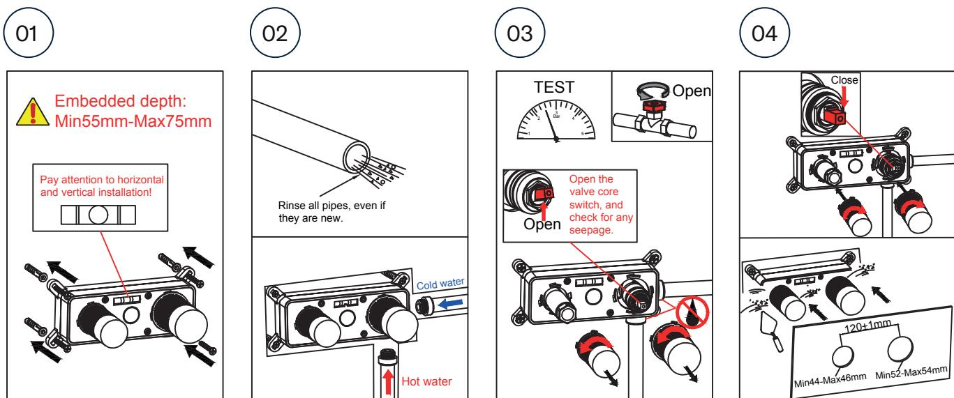
DIG THE EMBEDDED HOLE IN THE WALL, THE EMBEDDED DEPTH IS MIN55MM-MAX75MM. (NOTE:DEPTH DIMENSION IS REFERS TO THE WALL WITH PAVED TILE, AND PLEASE RESERVE APPROPRIATE TILE THICKNESS IF INSTALLED ON THE BLANK WALL). INSTALL THE EMBEDDED BOX INTO THE EMBEDDED HOLE WITH EXPANSION RUBBER PARTICLES AND SELF-TAPPING SCREWS, AND CHECK WHETHER THE LEVEL IS LEVEL.
