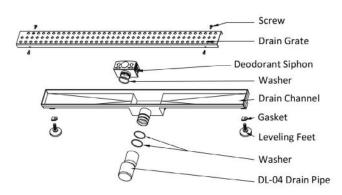
Determine the desired position of the shower drain. Relocate rough-in pipework if necessary. Cover with flooring mortar as needed.
