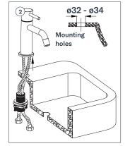
CONNECT THE WATER NOZZLE TO THE BASIN ACCORDING TO THE DRAWING, COMPLETE THE FIXING SET, AND PUT THE SECOND INLET PIPE INTO THE MAIN BODY
