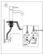
CONNECT THE TWO INLET HOSES TO THE ANGLE VALVE, WHICH FROM THE MAIN BODY OF THE FAUCET, ACCORDING TO THE "RED", "BLUE" INDICATED ON THE FAUCET HANDLE, AND CONNECT THE HOT AND COLD WATER SEPARATELY.
