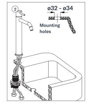
CONNECT THE WATER NOZZLE TO THE BASIN ACCORDING TO THE DRAWING, COMPLETE THE FIXING SET, AND PUT THE SECOND INLET PIPE INTO THE MAIN BODY
