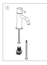
ACCORDING TO THE ABOVE DRAWING, BEFORE THE HOSE IS INSTALLED, DISTINGUISH LEFT RED (HOT WATER) AND RIGHT BLUE (COLD WATER).
