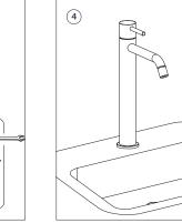
AFTER INSTALLATION, SWING THE OUTLET PIPE FROM SIDE TO SIDE AND TEST WHETHER EACH CONNECTION IS LEAKINGOR NOT.
