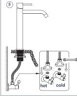
CONNECT THE TWO INLET HOSES TO THE ANGLE VALVE, WHICH FROM THE MAIN BODY OF THE FAUCET, ACCORDING TO THE "RED", "BLUE" INDICATED ON THE FAUCET HANDLE, AND CONNECT THE HOT AND COLD WATER SEPARATELY.
