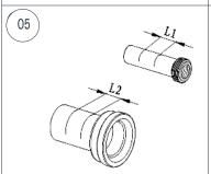
AS PER DRAWING, L1 IS DISTANCE BETWEEN THE TWO LINES ON STRAIGHT TUBE. L2 IS DISTANCE BETWEEN THE TWO LINES ON CONNECTING PIPE.
