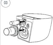
APPLY LUBRICANT ON RUBBER WASHERS OF STRAIGHT TUBE AND CONNECTING PIPE, THEN CERAMIC HOLES.
