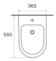
Due to the simplicity of the back-to-wall concept. Installation is achieved by connecting the water inlet/outlet and securing the bidet with the included fixing kit.
