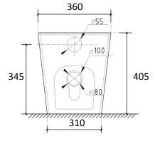
Due to the simplicity of the back-to-wall concept. Installation is achieved by connecting the water inlet/outlet with the flushing mechanism and securing the WC with the included fixing kit.
