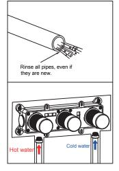
RINSE ALL PIPES, CONNECT THE COLD AND HOT WATER PIPES, PAYING ATTENTION TO DISTINGUISHING THE DIRECTION OF THE COLD AND HOT WATER PIPES.
