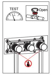
TAKE OUT THE ROUND COVER OF THE EMBEDDED BOX, OPEN THE WATER VALVE SWITCH, CHECK IF THE VALVE IS IN A CLOSED STATE. AND CHECK FOR ANY SEEPAGE.
