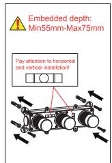
DIG THE EMBEDDED HOLE IN THE WALL, THE EMBEDDED DEPTH IS MIN55MM-MAX75MM. (NOTE: DEPTH DIMENSION IS REFERS TO THE WALL WITH PAVED TILE, AND PLEASE RESERVE APPROPRIATE TILE THICKNESS IF INSTALLED ON THE BLANK WALL).INSTALL THE EMBEDDED BOX INTO THE EMBEDDED HOLE WITH EXPANSION RUBBER PARTICLES AND SELF-TAPPING SCREWS, AND CHECK WHETHER THE LEVEL IS LEVEL.
